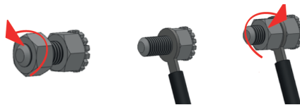
Fig. 4 Connecting the device to an electrical equipotential bonding system
